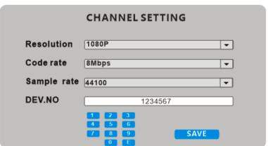
Resolution: DVR auto detect input signal in 1080P(1920x1080),720P(1280x720) resolution
